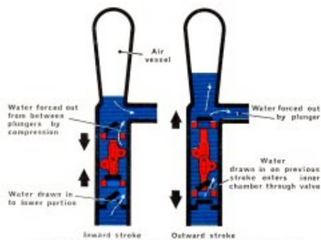
Fig. 1-6. Diagram showing the operation of one type of double-acting lift pump.
